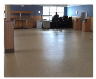
The Dining Hall received an upgrade of new flooring. The concrete was covered with an epoxy making it easier to clean. We think it looks better too! We have also added AC and heat pumps for more energy efficiency!
